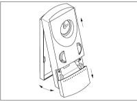
Feed the connection wires through the opening in the unit's base
