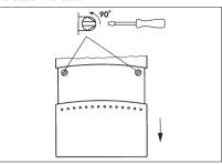
Remove the room thermostat clock from its base
